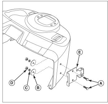
Figure 16. Mount Control Bracket - Current Models
